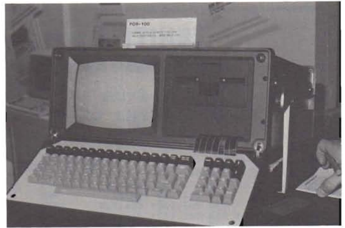
The POR-100 from Kres Engineering. It is a Z-100 installed in a transportable case.
